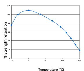
"Hot strength" shear strength tests performed on mild steel. 24hr cure at room temperature and conditioned to pull temperature for 30 minutes before testing.
