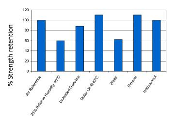
Specimens were immersed for 1000 hours at 22  $^{\circ}$ C (unless otherwise stated).
