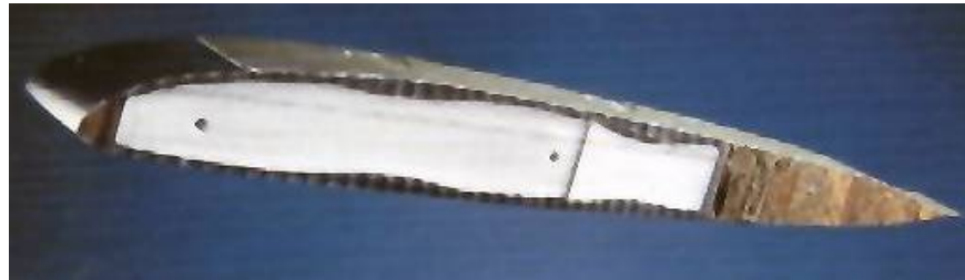
Cross-section of main rotor blade of the EH 101 with a ROHACELL® core
