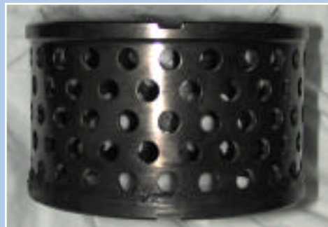
JT8D-219 #4 Squirrel Cage 10,700+ hours on BPTO 2197
