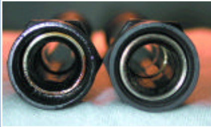
JT8D-219 #4 Oil Pressure/Scavenge Tube 10,700+ hours on BPTO 2197
