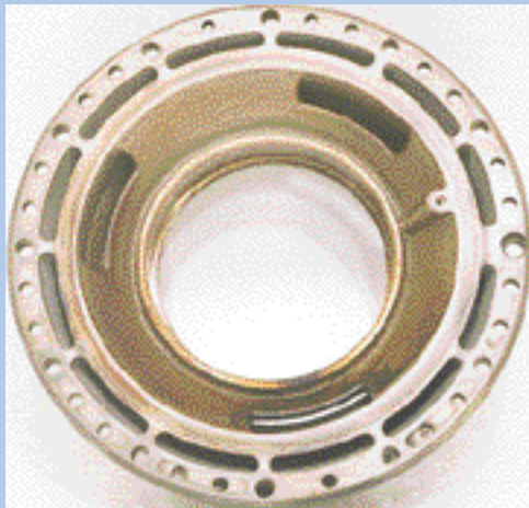
TSCP700 APU Turbine Bearing Compartment 1600+ hours on BPTO 2197
