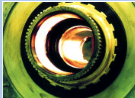
JT8D-219 Center Tube 8600+ hours on BPTO 2197
